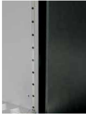
Safety optical barrier (light curtain) in Class 2 (only for Plus)
